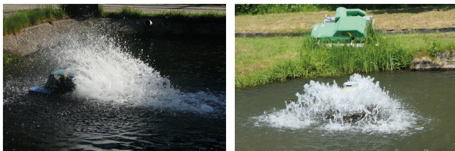
Figure 1: Various types of aerators to ensure adequate oxygen supply in rainbow trout rearing units, photos: © Thünen Institute / Vincent Lugert.
